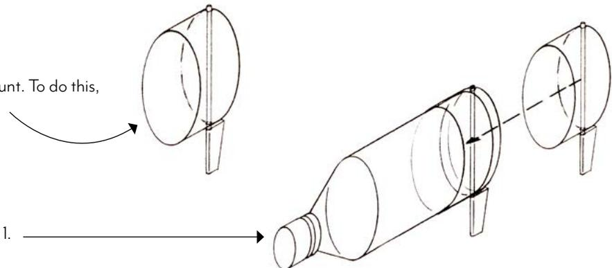
5. Slide the rudder and rudder mount onto bottle 1.
