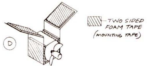
6. Cut mounting tape and place it around three sides of the motor and two surfaces of the mount and place the motor into the mount.
