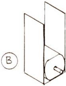
3. Bend and slightly fold the sides up and around the motor.
