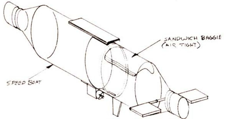
4. Punch two holes, one on either side of the neck of the bottle you took the bottom off of, and run the shaft through these two holes. If you're confused, look at the image above this step.
