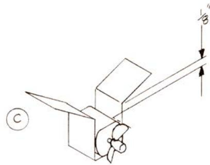
4. Place the propeller onto the motor shaft to figure out the clearance from the top of the prop to the bottom of bottle 1.
