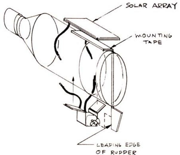
1. Use the one **gray** wire nut to connect the **blue** wire from the solar array to the **red** wire of the motor.
