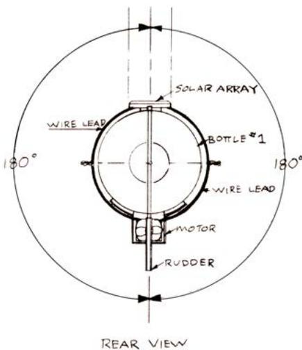
2. After the motor and rudder are aligned, mount the solar array.
